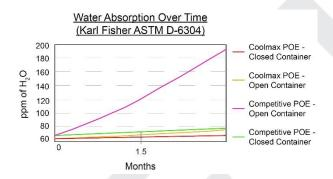
Even in an open container Coolmax POE has shown to absorb less water then most competitive PEO fluids
