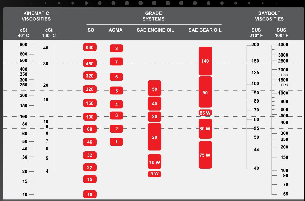
Viscosities can be related horizontally only. For example, the following oils have similar viscosities: ISO 460, AGMA 7 and SAE GEAR OIL 140. The viscosity/temperature relationships are based on 95 VI oils and are usable only for mono grade engine oils, gear oils and other 95 VI oils. Crankcase oils and gear oils are based on 100° C viscosity. The "W" grades are classified on low temperature properties. ISO oils and AGMA grades are based on 40° C viscosity.
